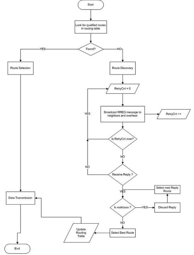
Figure 3: Trusted Routing Algorithm
