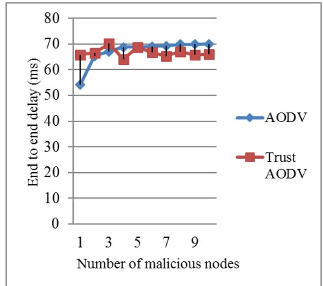
Figure 6: End to end delay vs number of malicious nodes.
