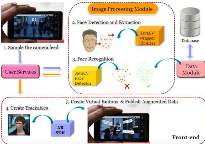
Fig.5. - Augmented Identification Module Overview
